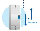
Set the circuit breaker to O, wait for 5 seconds, and then set the circuit breaker back to I. This manoeuvre is equivalent to pressing the + button on the meter and is understood by the meter as an instruction to close the breaking component.
